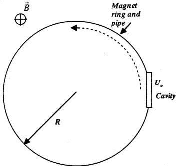
This procedure is repeated, causing the particle to steadily gain energy. The magnetic field is increased each orbit to keep the orbit radius constant at R.
